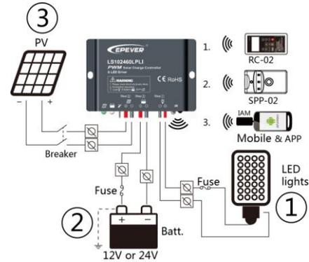
Figure 2 Wiring
